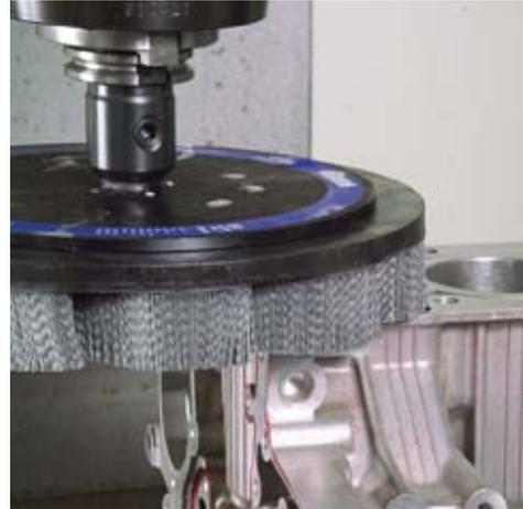
*Osborn's ATB (Advanced Technology Brushing) abrasive filament brushes engineer abrasive nylon into flexible tools for highly refined finishing processes.*
